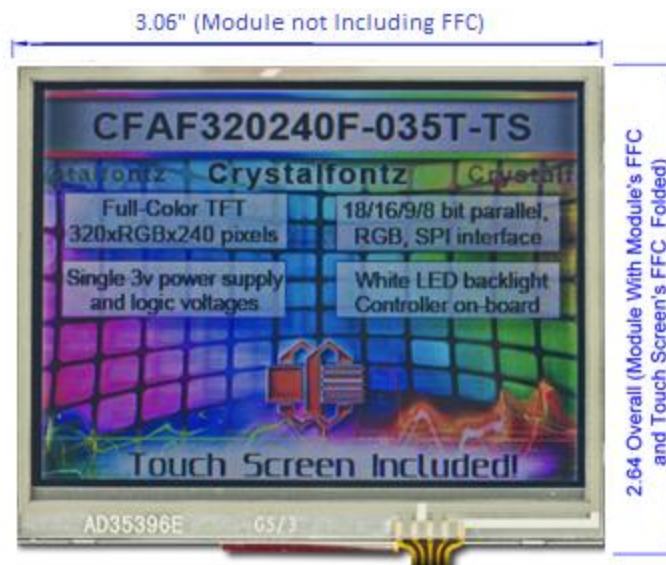
Figure 32: Crystalfontz CFAF320240F-035T-TS - Unmodified, Appears as the Camera Perceives the Display (showing no FPC connectors)
