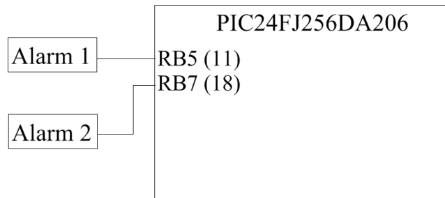
Figure 13: Interfacing Alarm Outputs with the PIC24FJ256DA206
