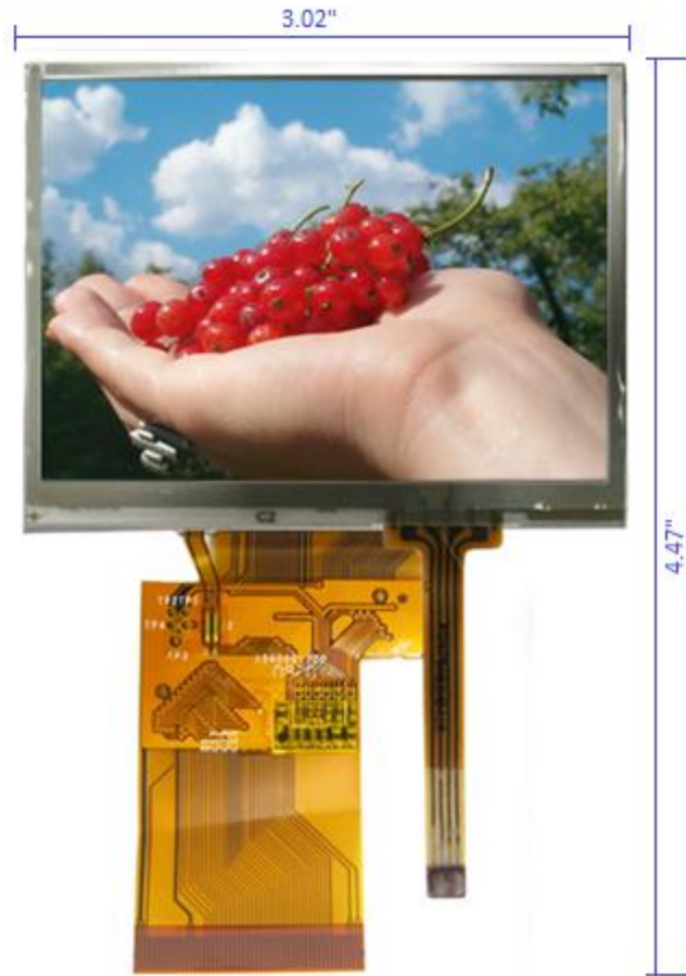
Figure 34: Newhaven NHD-3.5-320240MF-ATXL#-T-1 Display (showing FFC connectors)
