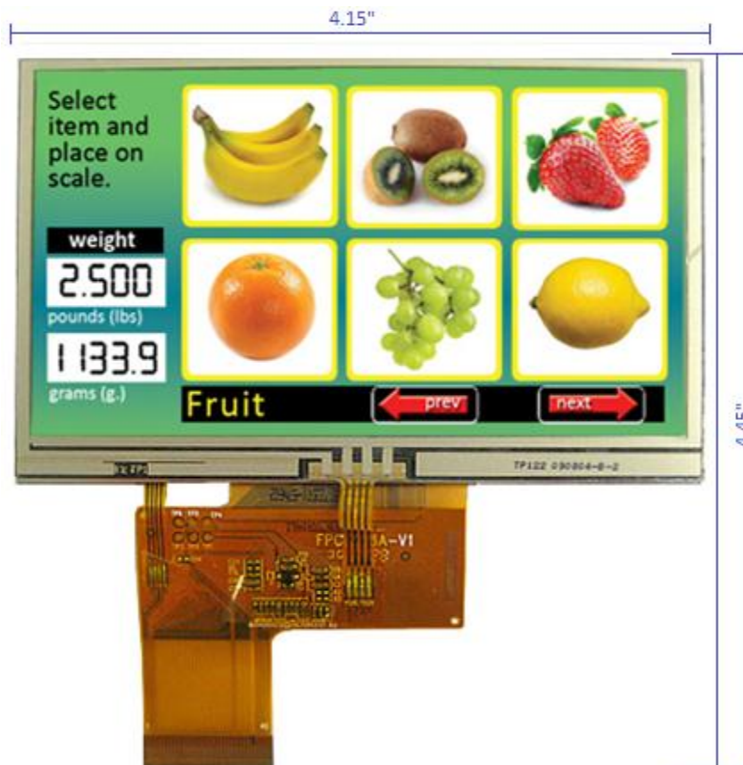
Figure 33: Newhaven NHD-4.3-480272MF-ATXI#-T-1 Display (showing FFC connectors)
